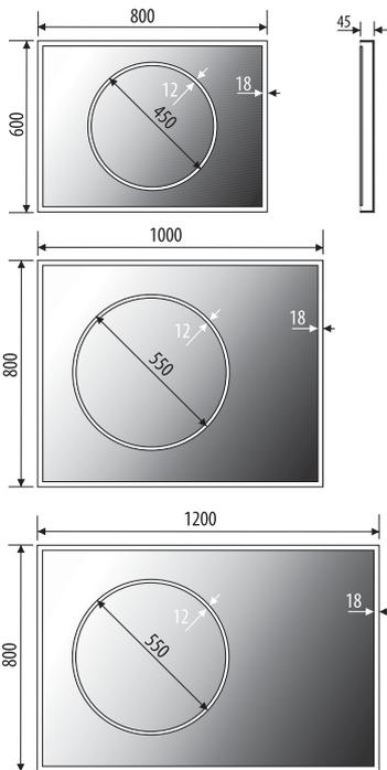
4mm mirror, construction - varnished steel
